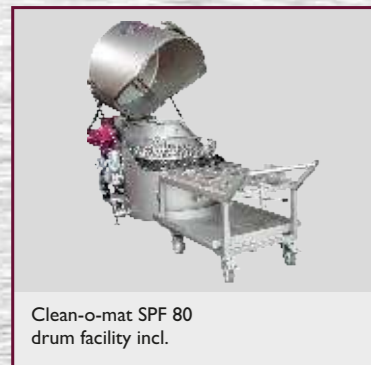
Clean-o-mat SPF with loading platform and rotating basket
